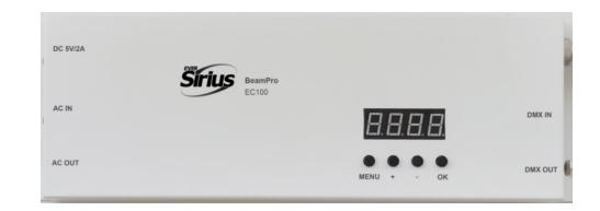
**3. DMX address setting**. Press the "MENU" button on the controller until you see "A\*\*\*" (\* stands for a number) in the LCD, and press "+" or "-" button to select an address for the EC100 panel.
